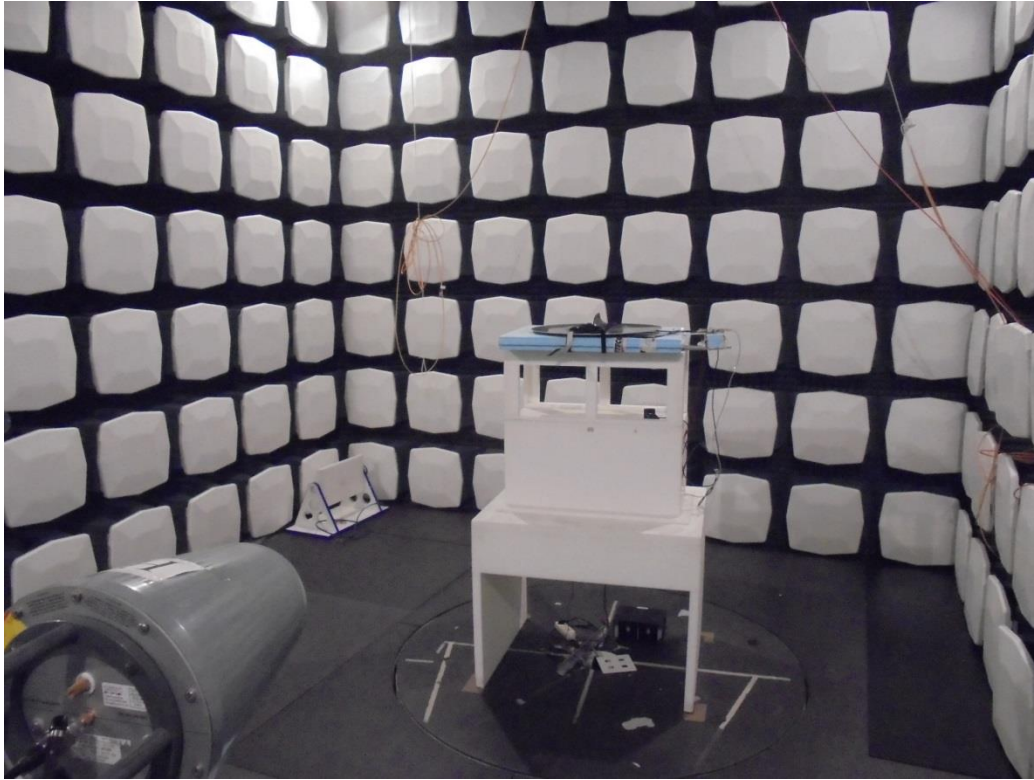
Photograph 1: Radiated field strength measurements in FAR (Fully Anechoic Chamber)
