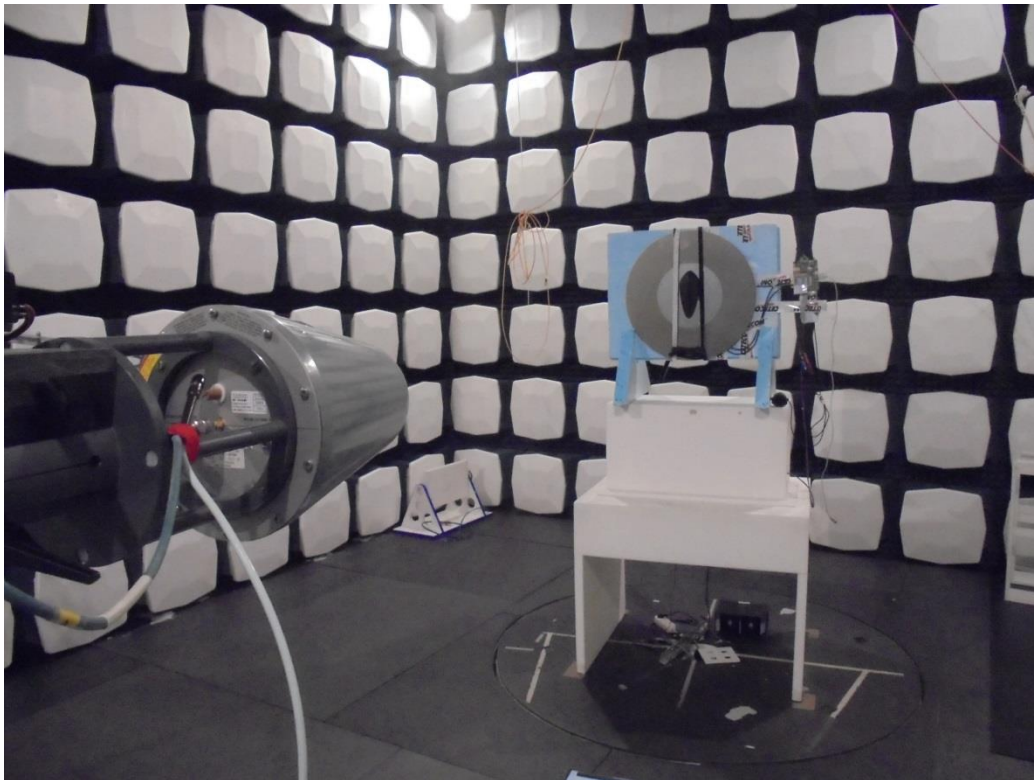
Photograph 2: Radiated field strength measurements in FAR (Fully Anechoic Chamber)
