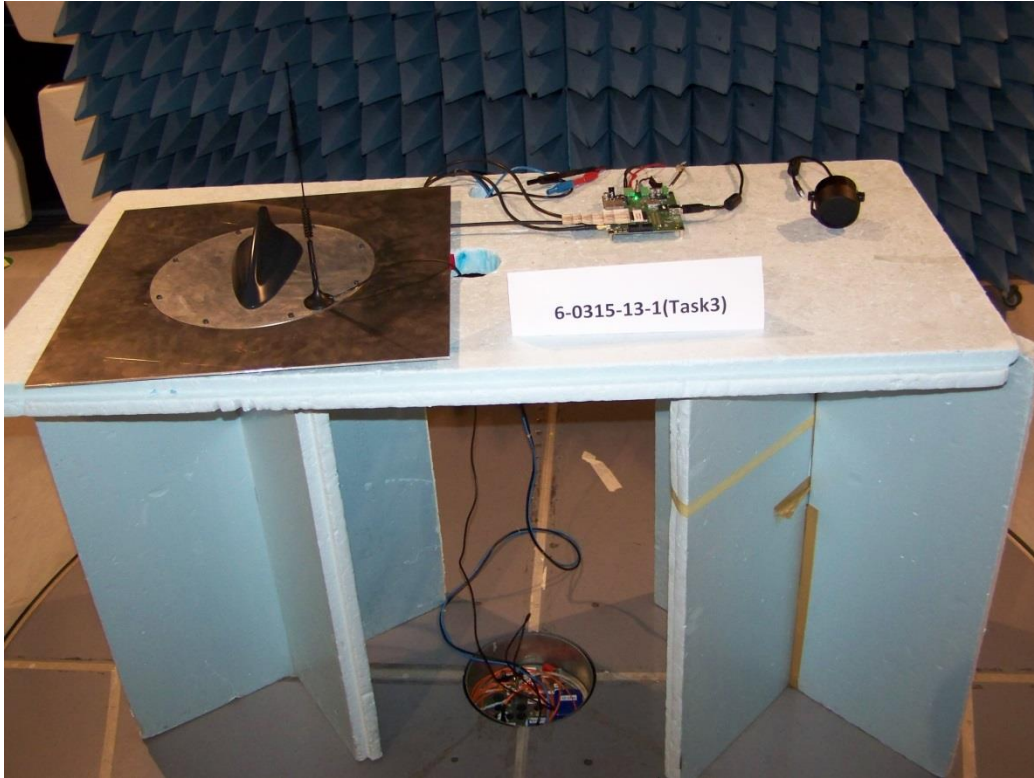
Photograph 3: Radiated field strength measurements in SAR (Semi Anechoic Chamber)
