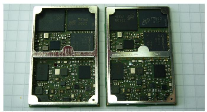
Fig. 1: The right module shows the old shield frame, the left module the new shield frame with increased height
