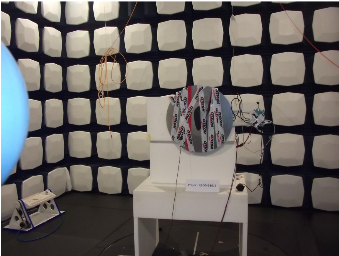
Photograph 1: Measurements in fully-anechoic chamber (EUT vertical position)
