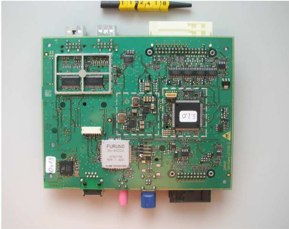
Main PCB bottom view (metal shield removed)
