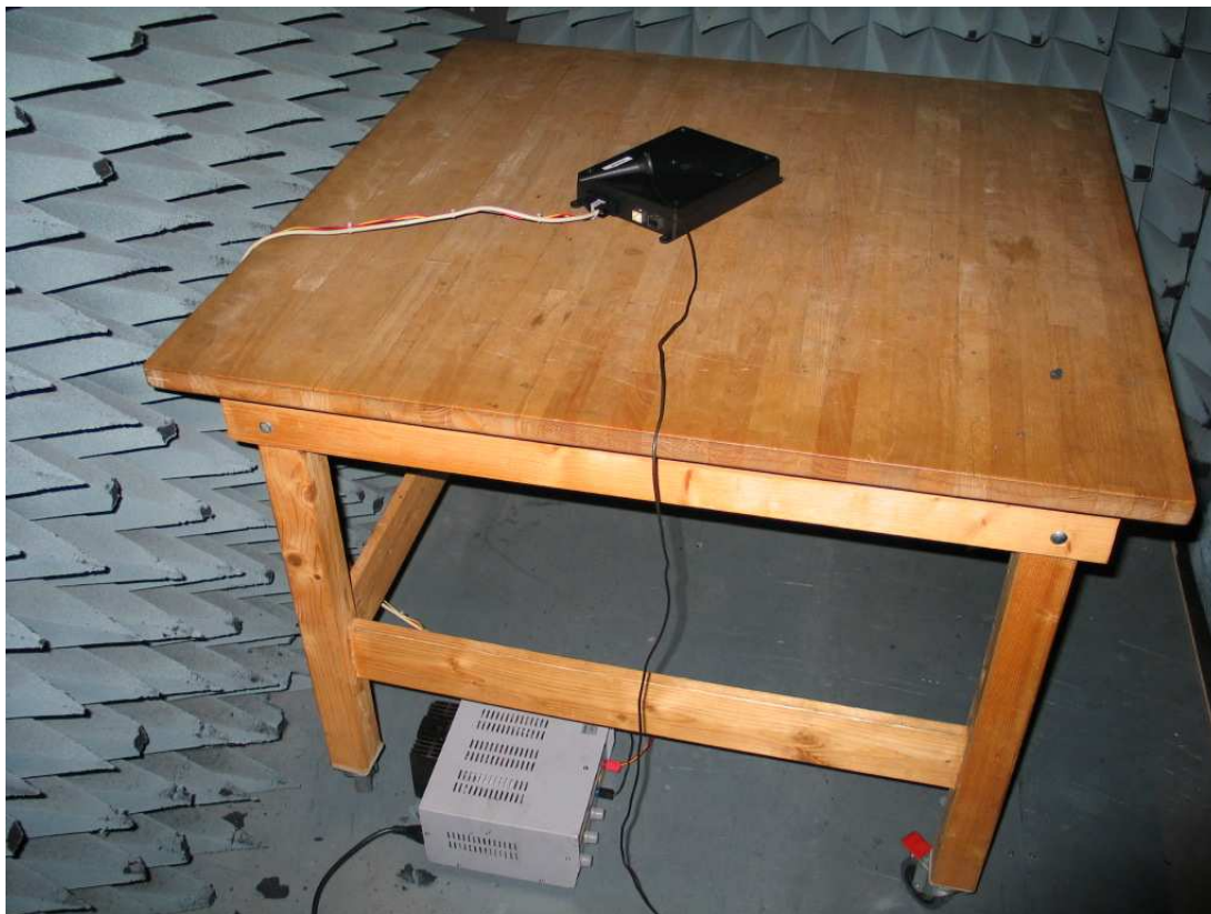
Photo 3: Test setup for radiated measurements (below 30MHz)
