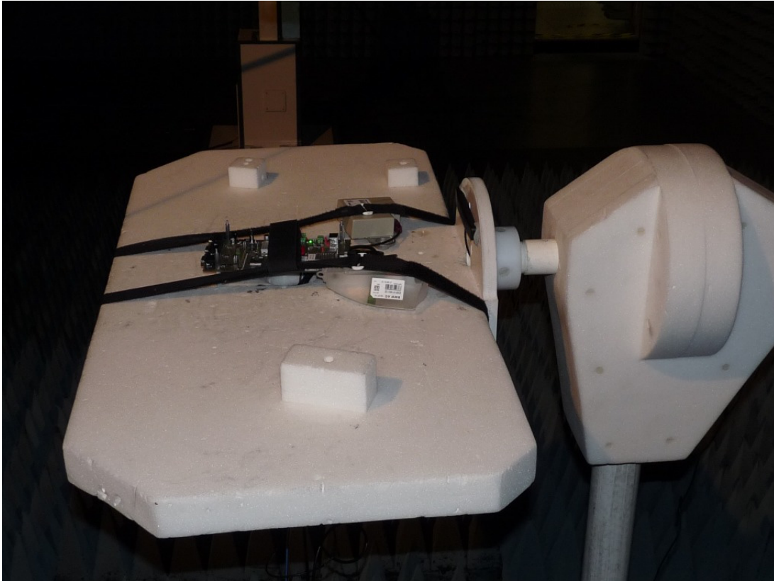
Photo 1: Test setup for radiated tests, spurious emissions acc. to FCC Part 22, 24 and IC RSS-Gen (above 1 GHz)
