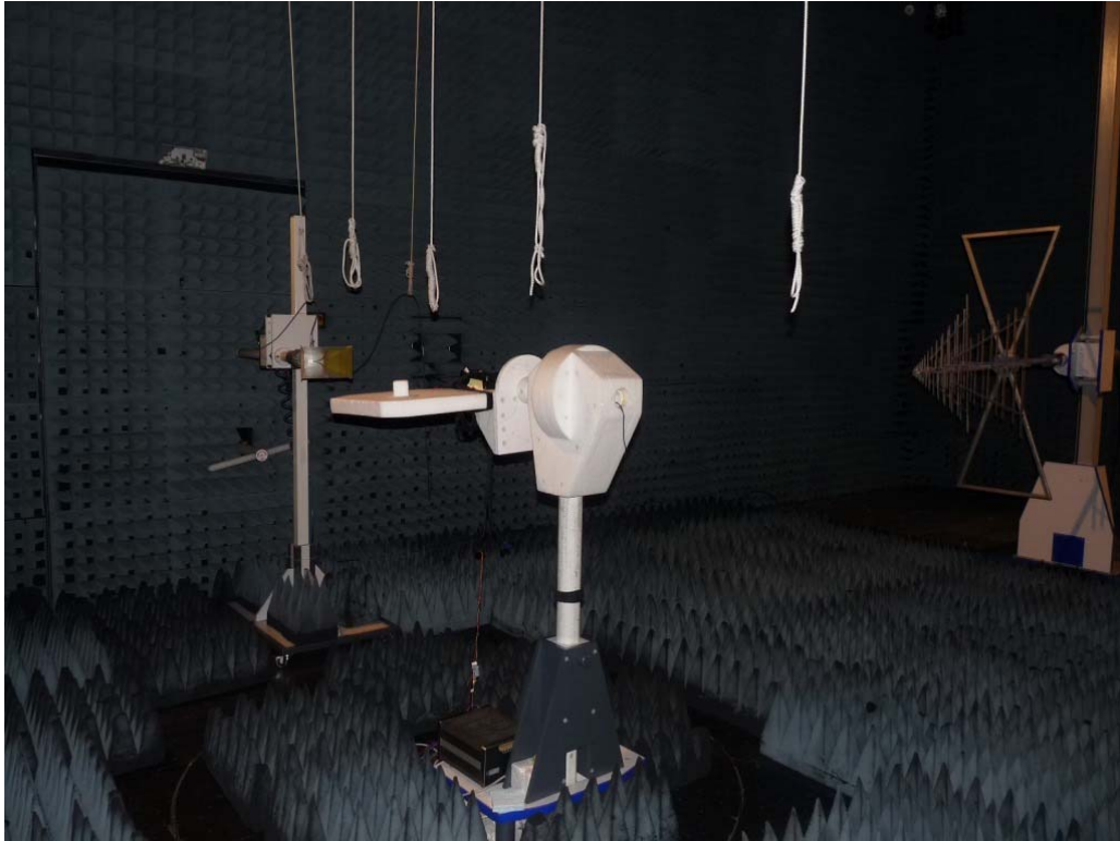
Photo 4: Test setup for spurious radiated emissions measurements (Enclosure, full-equipped anechoic chamber, 1 GHz -1.8GHz intentional radiator §15)
