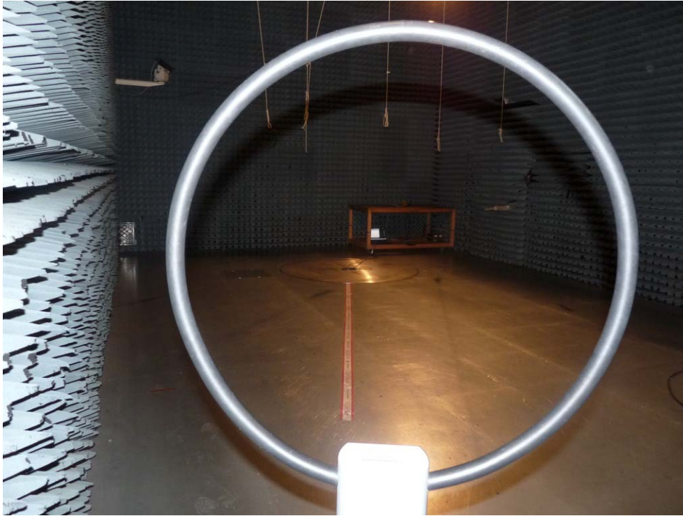
Photo 1: Test setup for spurious radiated emissions measurements (Enclosure, semi-anechoic chamber, 9 kHz to 30 MHz, unintentional radiator §15)
