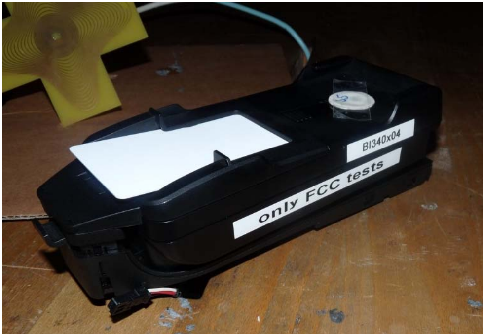
Photo 2: The EUT on the table shown at Photo 1 for spurious radiated emissions measurements (Enclosure, semi-equipped anechoic chamber, 9 kHz to 30 MHz, unintentional radiator §15)
