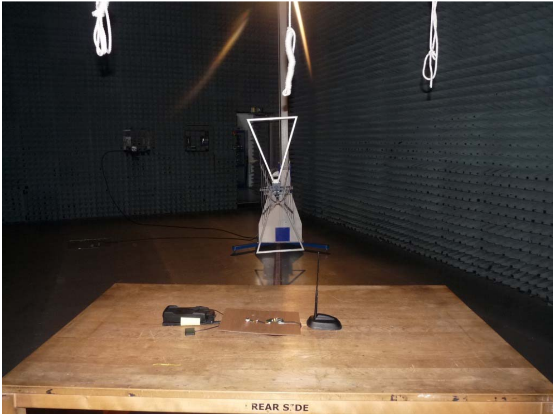
Photo 3: Test setup for spurious radiated emissions measurements (Enclosure, semi-equipped anechoic chamber, 30 MHz -1GHz intentional radiator $15)
