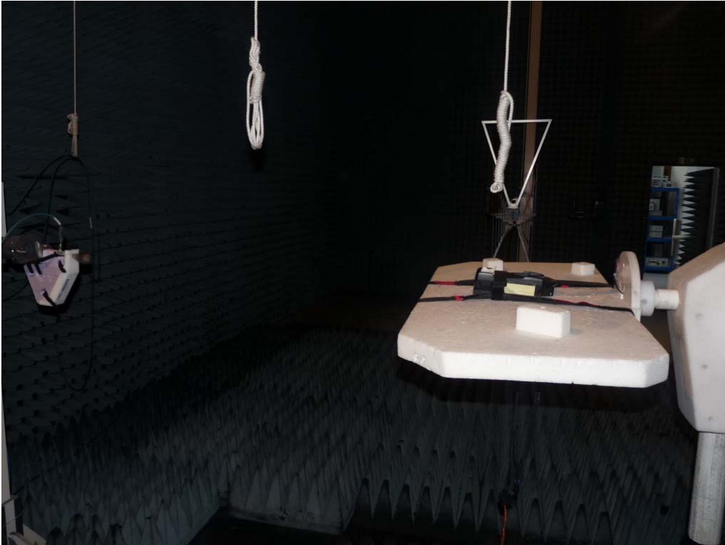
Photo 5: Test setup for spurious radiated emissions measurements (Enclosure, full-equipped anechoic chamber, 1 GHz -25GHz intentional radiator §15)
