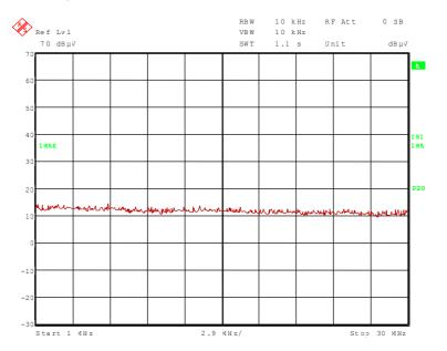
No significant frequencies above the noise floor of the system were found during the preliminary radiated emission test inside this frequency range, so no measurements were carried out on the outdoor test site.
