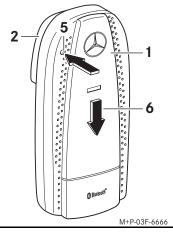
Press and hold the release button (5). Slide the Mercedes-Benz Cradle adaptor with Bluetooth<sup>®</sup> (1) in direction of arrow (6) and remove it from the pre-installed contact plate (2).
