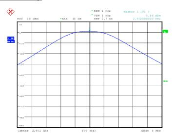
113907\_10.wmf: Maximum peak output power at the middle of the assigned frequency band (operation mode 2):
