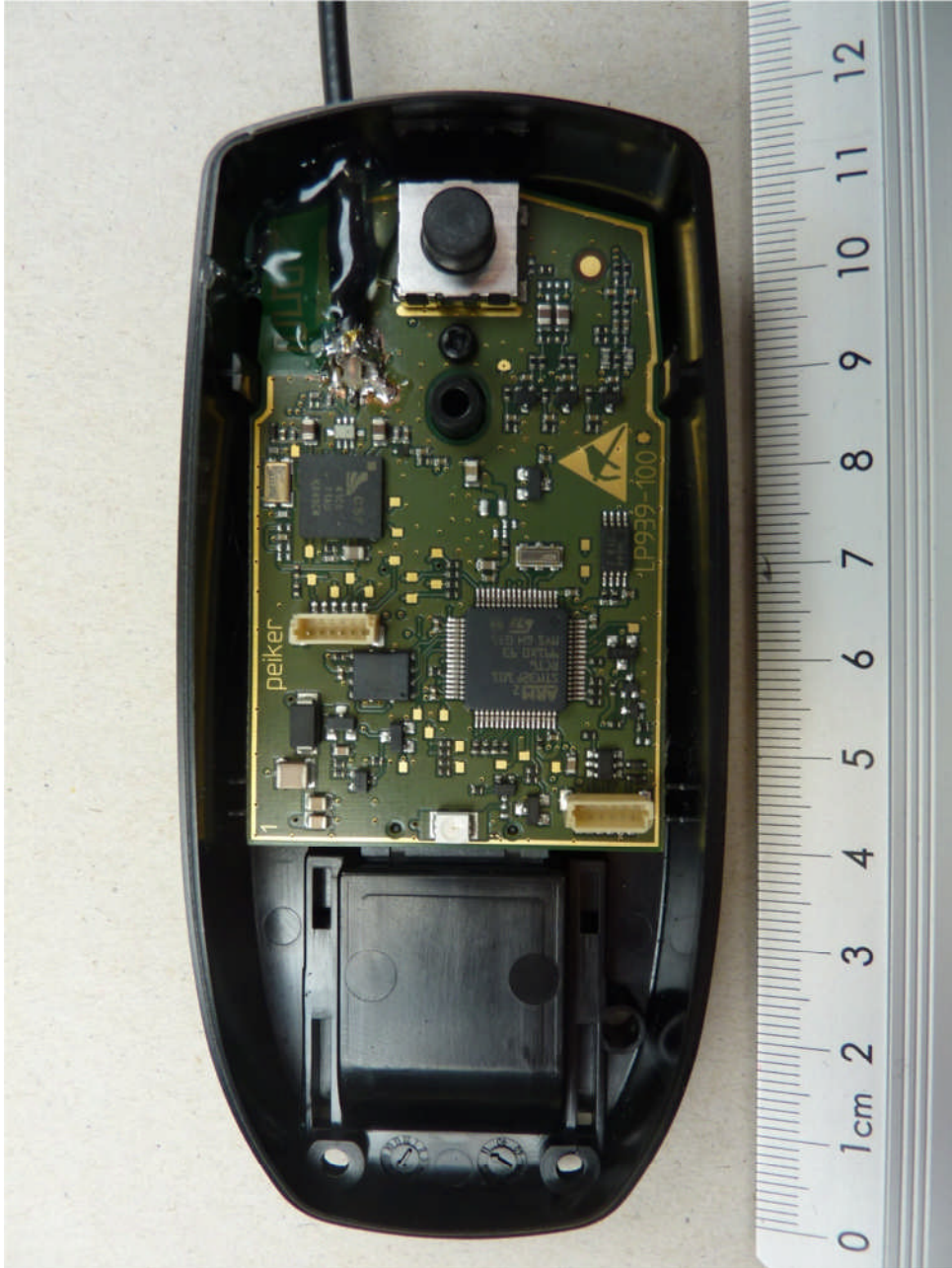
113907_05: CKIII-HFP4, internal view with temporary antenna connector
