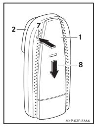
Press and hold the release button (6). Slide the Mercedes-Benz Cradle adaptor with Bluetooth<sup>®</sup> (1) in direction of arrow (7) and remove it from the pre-installed contact plate (2).
