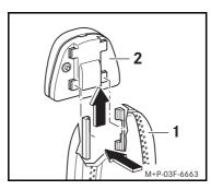
Insert the Mercedes-Benz Cradle adaptor with Bluetooth<sup>®</sup> (1) into the latches on the pre-installed contact plate (2), located in the center console. To insert the Mercedes-Benz Cradle adaptor with Bluetooth<sup>®</sup> (1), slide it upwards until it clicks into place.
