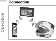
Telephone and navigation device cannot be connected with a helmet with a communication system at the same time. The telephone must be incorporated in the Bluetooth combination via the navigation device to enable both devices to be used at the same time. To do so, the navigation device is connected with the communication system as described (IIII 20). In addition, the telephone must be connected with the navigation device. The navigation device then announces, accepts and ends any phone calls.
