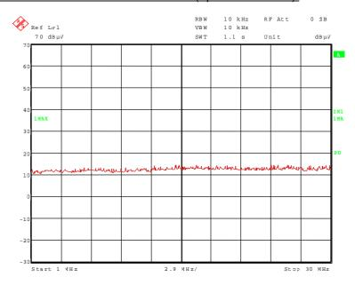
No significant frequencies above the noise floor of the system were found during the preliminary radiated emission test inside this frequency range, so no measurements were carried out on the outdoor test site.
