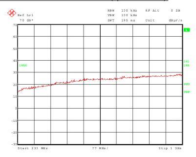
No significant frequencies above the noise floor of the system were found during the preliminary radiated emission test inside this frequency range, so no measurements were carried out on the open area test site.
