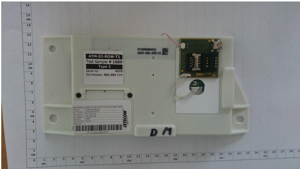
Photograph 7: Conducted Sample with external SIM CARD holder
