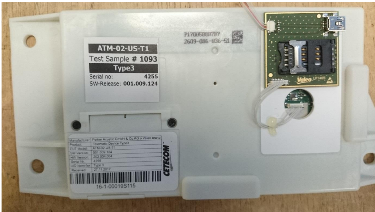
Photograph 7: Conducted Sample with external SIM CARD holder
