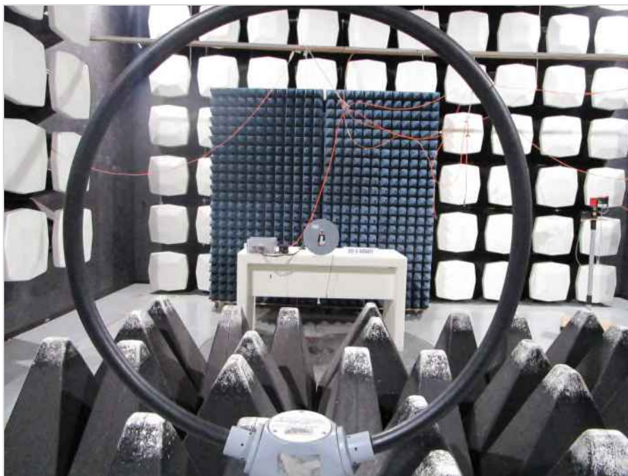
Photograph 4: EUT Test Setup in the semi anechoic chamber, overview
