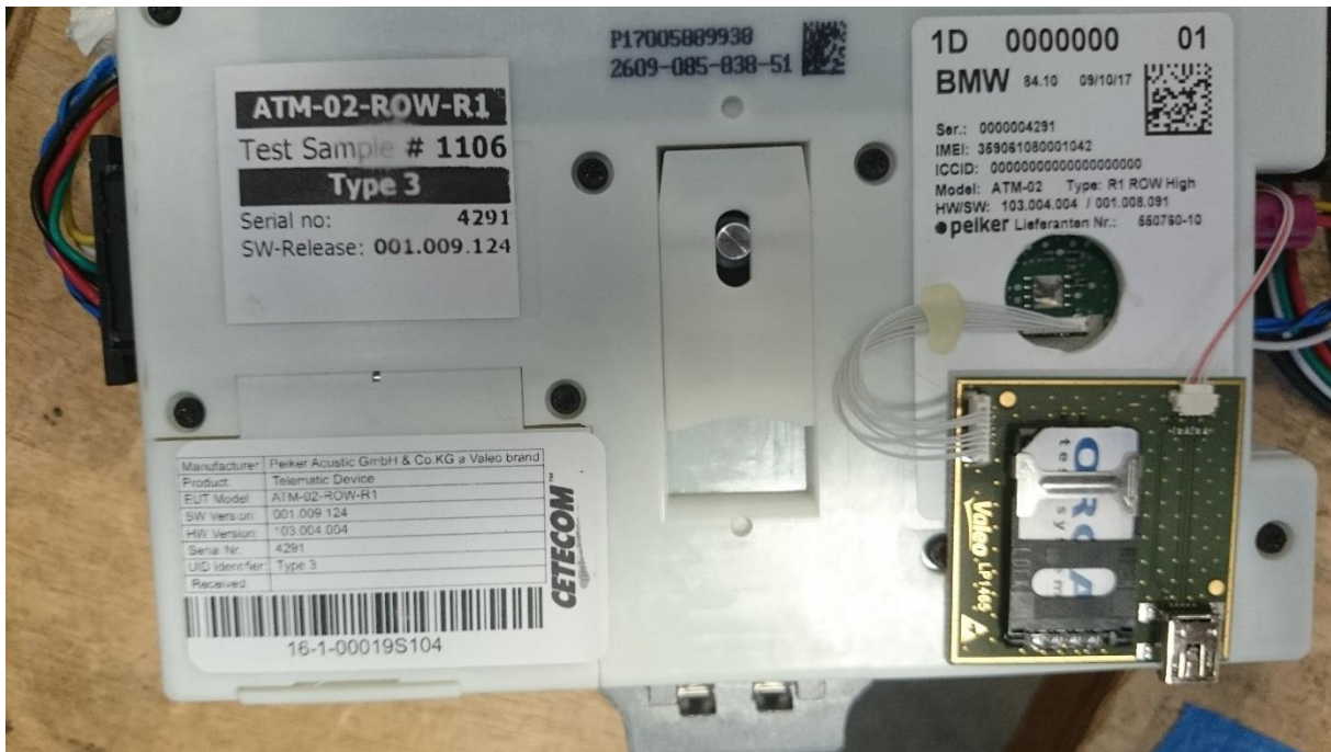
Photograph 7: Conducted Sample with external SIM CARD holder
