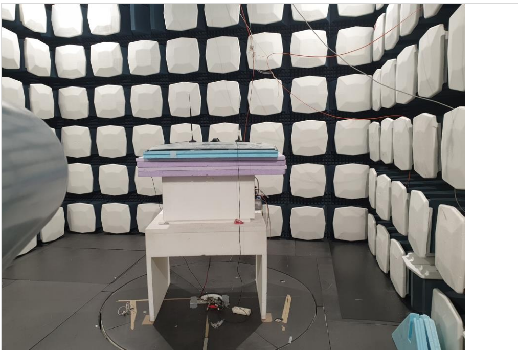
Photograph 4: EUT Test Setup 2 in the fully anechoic chamber, overview
