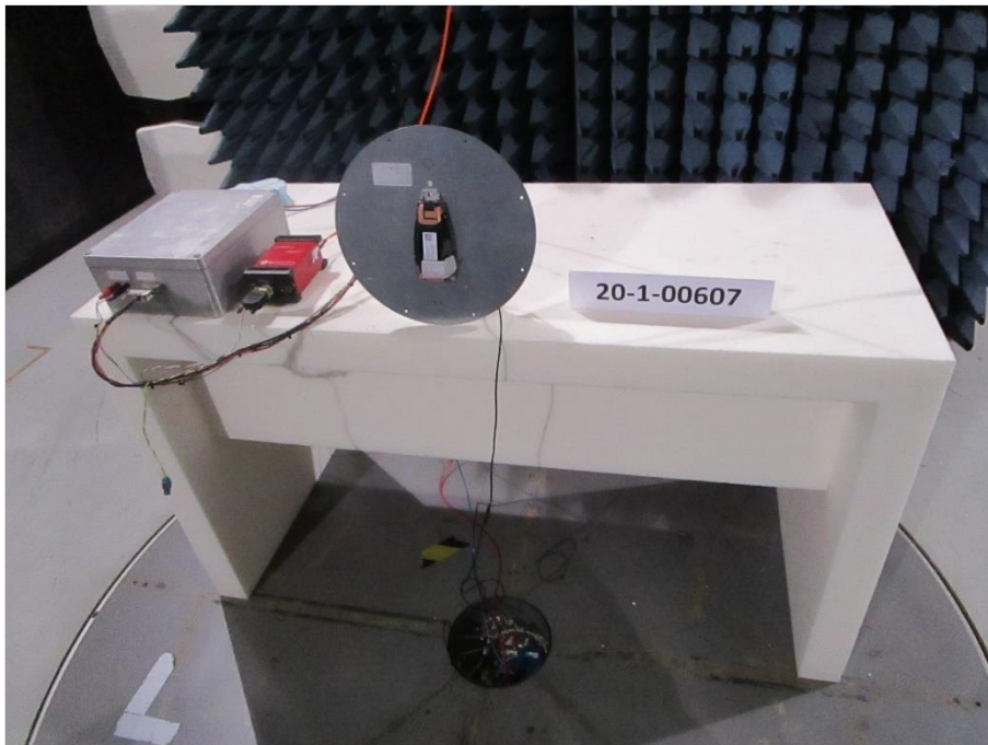
Photograph 5: EUT Test Setup in the semi anechoic chamber, close up view
