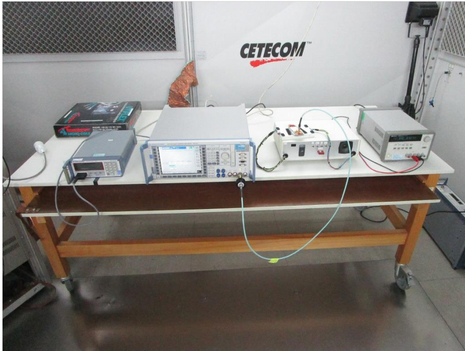
Photograph 7: EUT Setup 3 Conducted RF measurement
