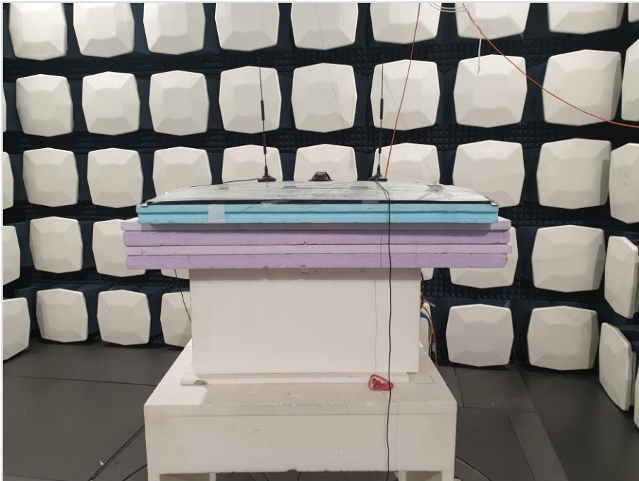
Photograph 3: EUT Test Setup 2 in the fully anechoic chamber, close up view
