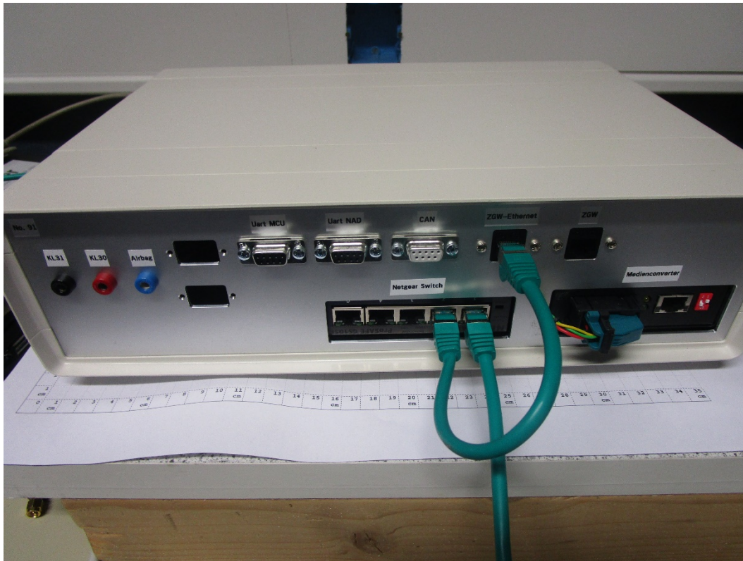
Photograph 10 Connectionbox inside chamber connected with laptop
