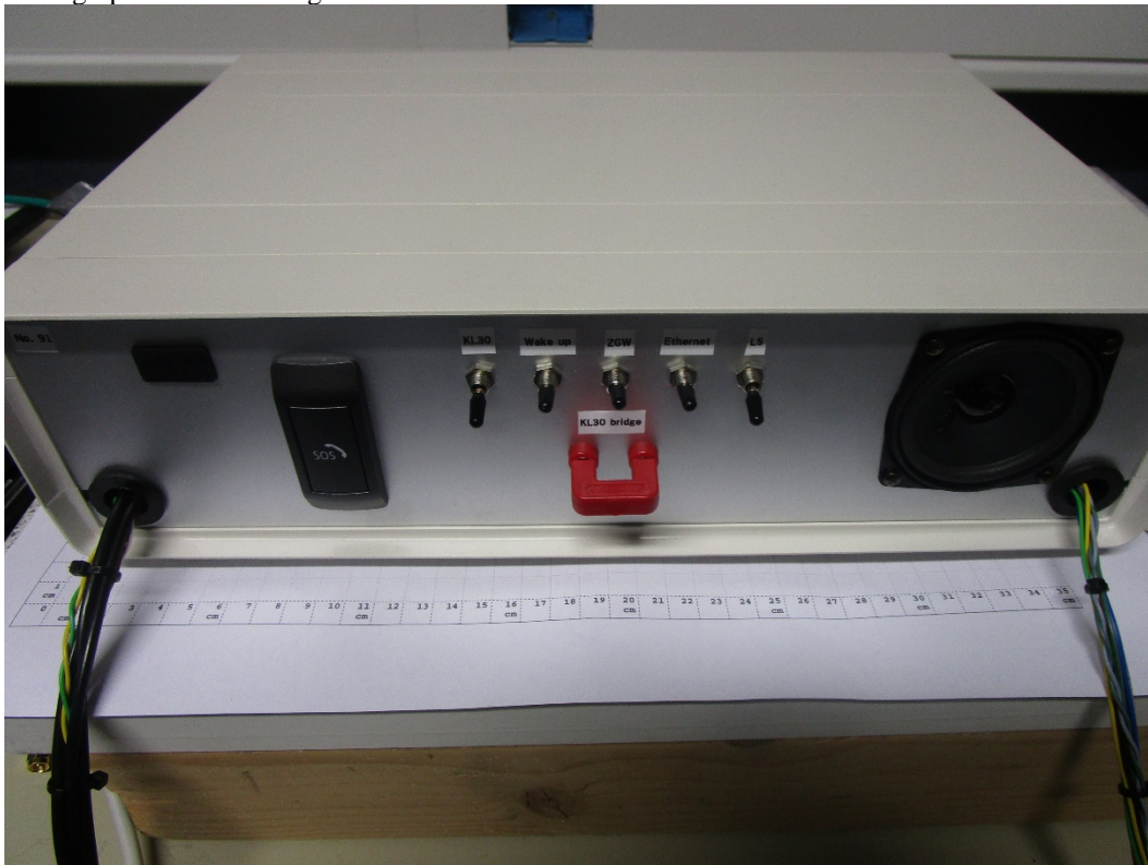
Photograph 9: connection box outside chamber
