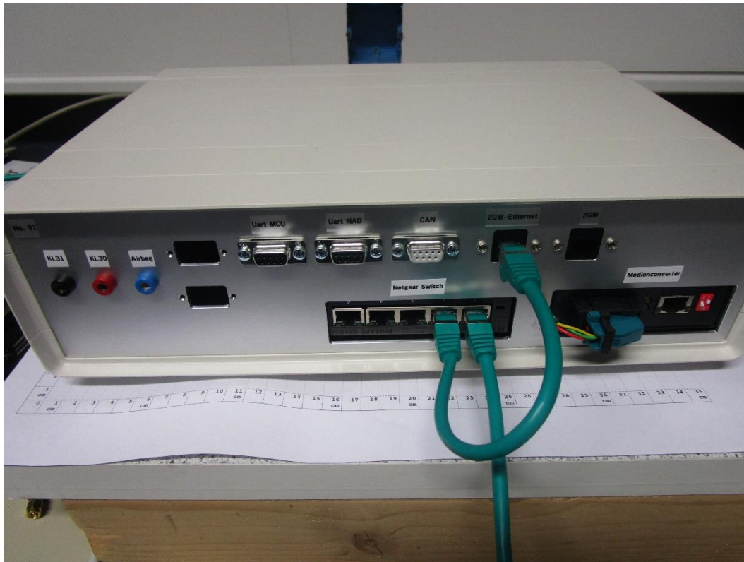
Photograph 12 Connectionbox inside chamber connected with laptop
