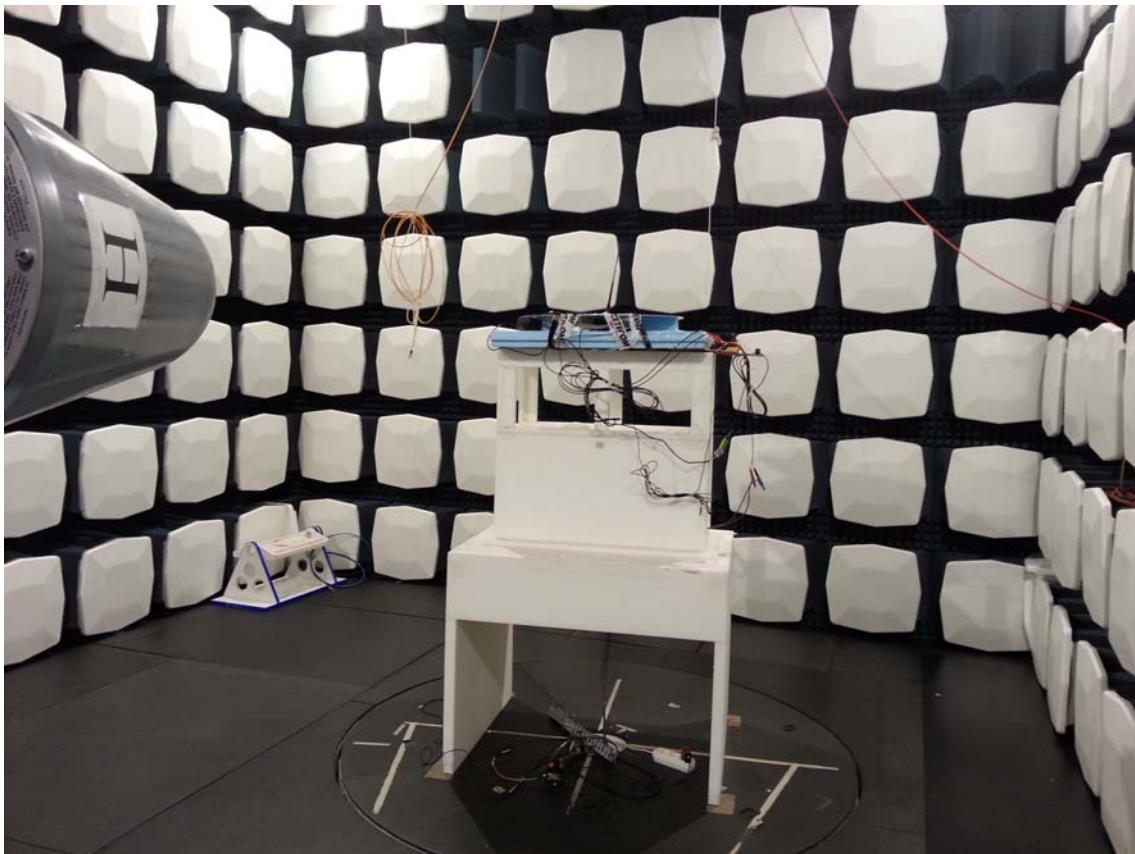
Photograph 2: Measurements in fully anechoic chamber (EUT A in horizontal position)
