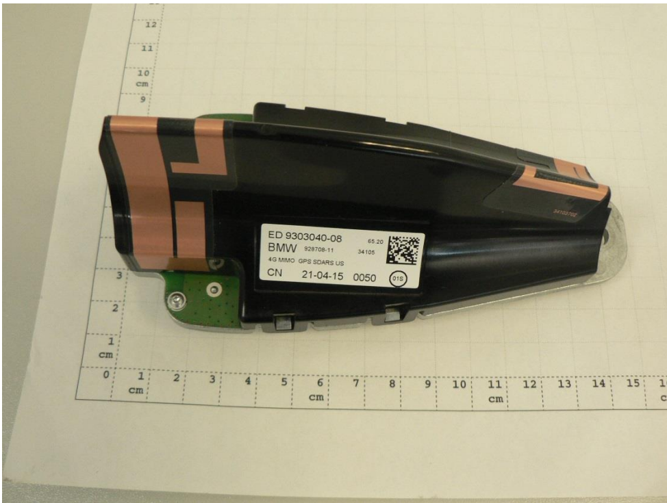
Photograph 8: Equipment under test: automotive roof pod
