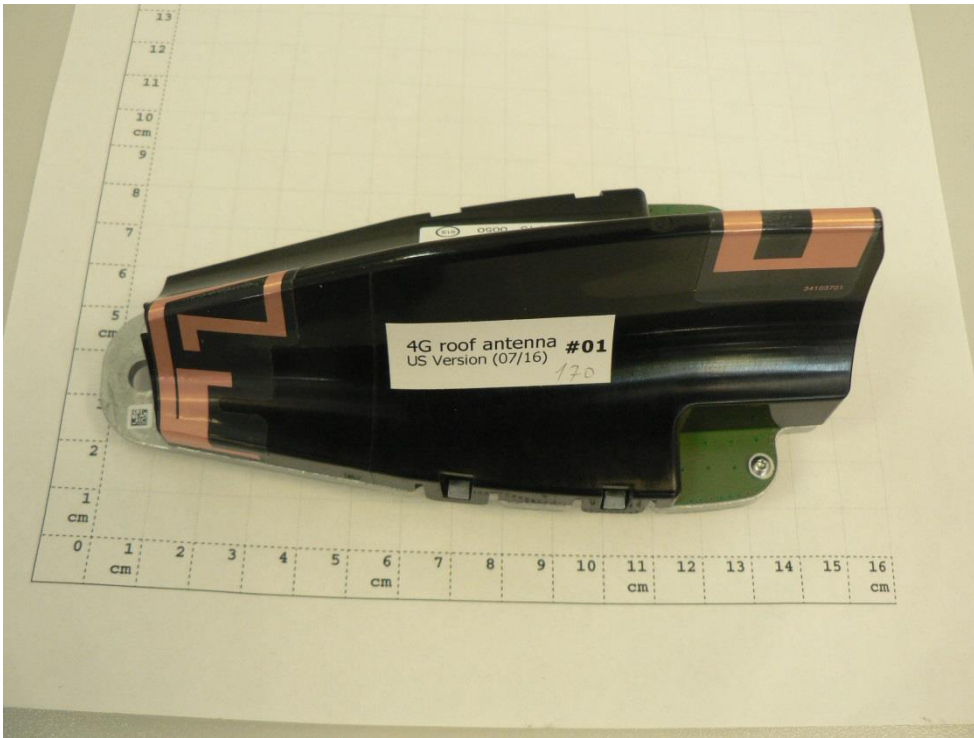
Photograph 7: Equipment under test: automotive roof pod
