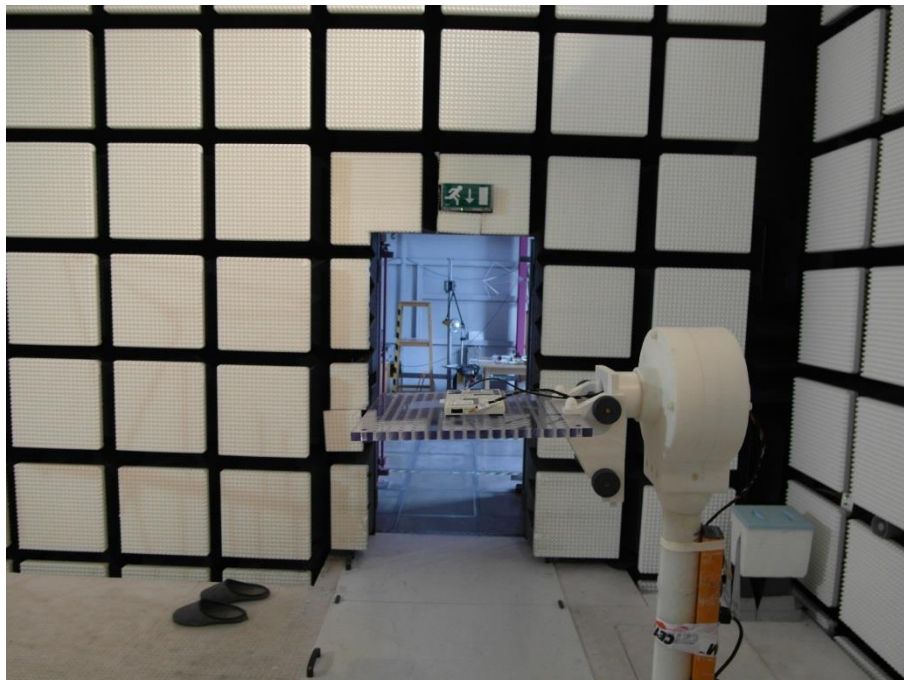
Photo 3: Test setup – internal antenna
