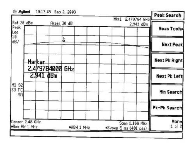
The Power (ERP) = Output power + cable loss + antenna gain = 2.941 dbm +1.7 db+ 0 dBi = 4.641 dbm
