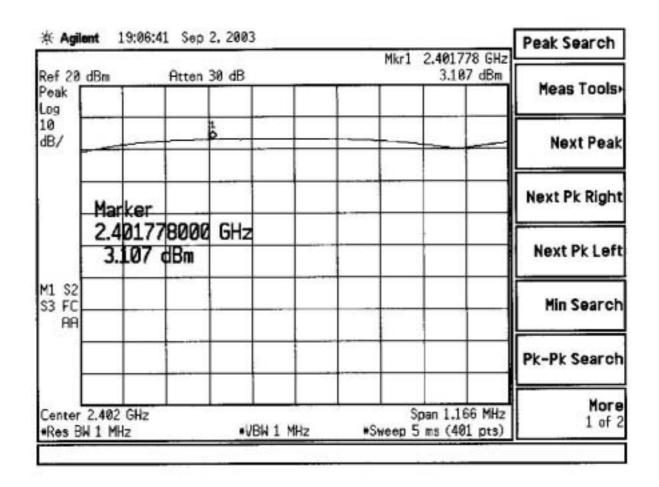
The Power (ERP) = Output power + cable loss + antenna gain = 3.107 dbm + 1.7 db+ 0 dBi = 4.8 dbm
