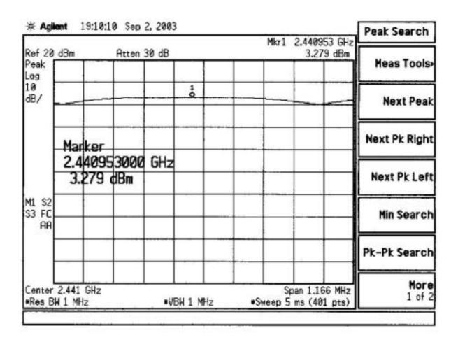
The Power (ERP) = Output power + cable loss + antenna gain = 3.279 dbm +1.7 db+ 0 dBi = 4.979 dbm
