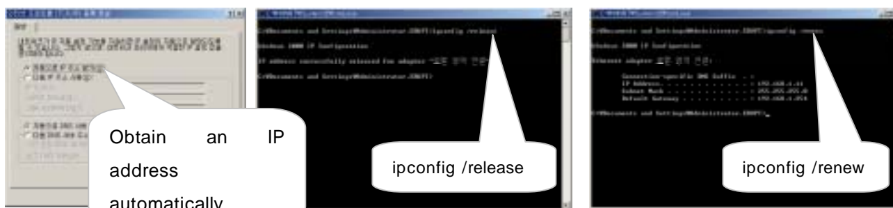
Setting Dynamic IP for using NasDisk - 2 Windows NT
