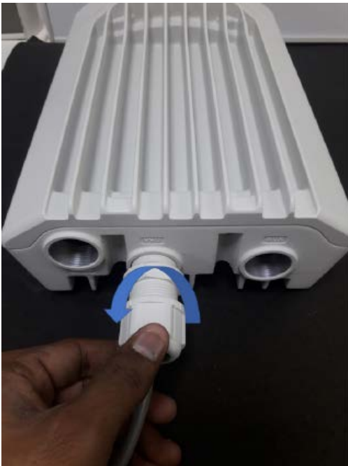
Figure 115: Removing the cable clamp
