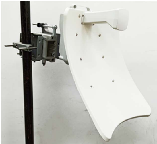
Figure 92: Locking the antenna alignment
