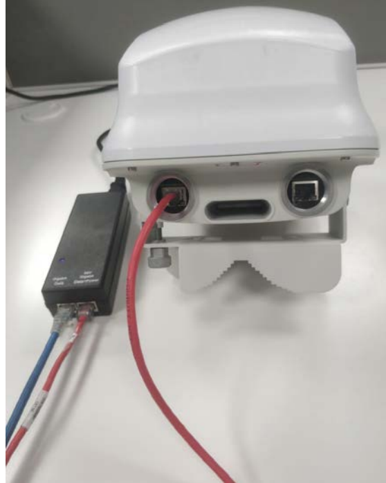
Figure 135: Connecting the V2000 power injector
