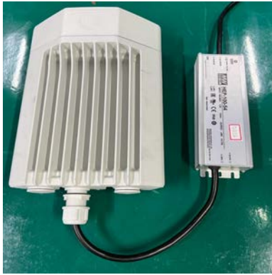
Figure 123: Connecting the output side of AC/DC PSU
