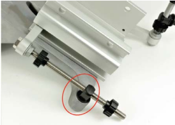
Figure 85: The pivot pin in the circular hole of mount
