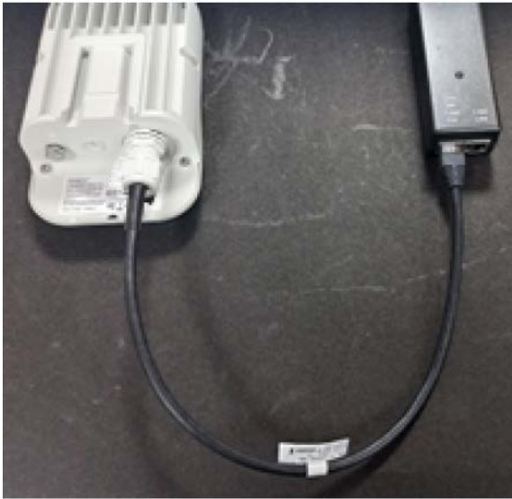
Figure 134: Connecting the V1000 Power injector
