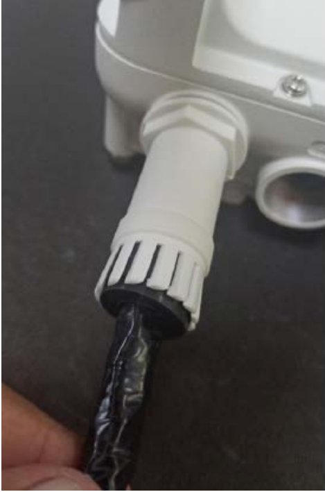
Figure 146: Fitting the gland body
