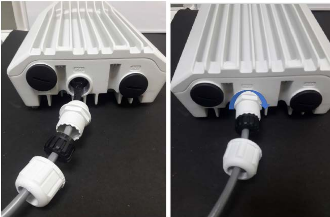
Figure 113: Connecting the RJ45 plug
