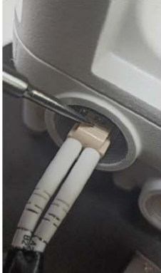
Figure 150: Pulling the bale clasp (latch)
