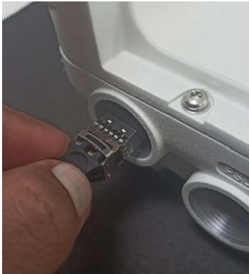
Figure 143: Rotating the latch
