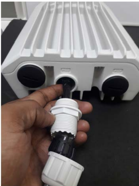
Figure 117: Removing the latch of the RJ45 plug
