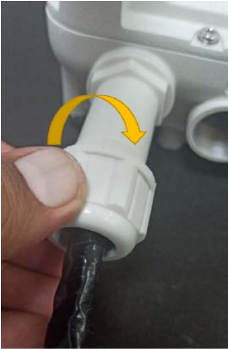
Figure 147: Fitting the gland nut
