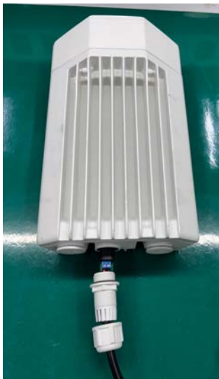
Figure 122: Connecting the input side of AC/DC PSU
