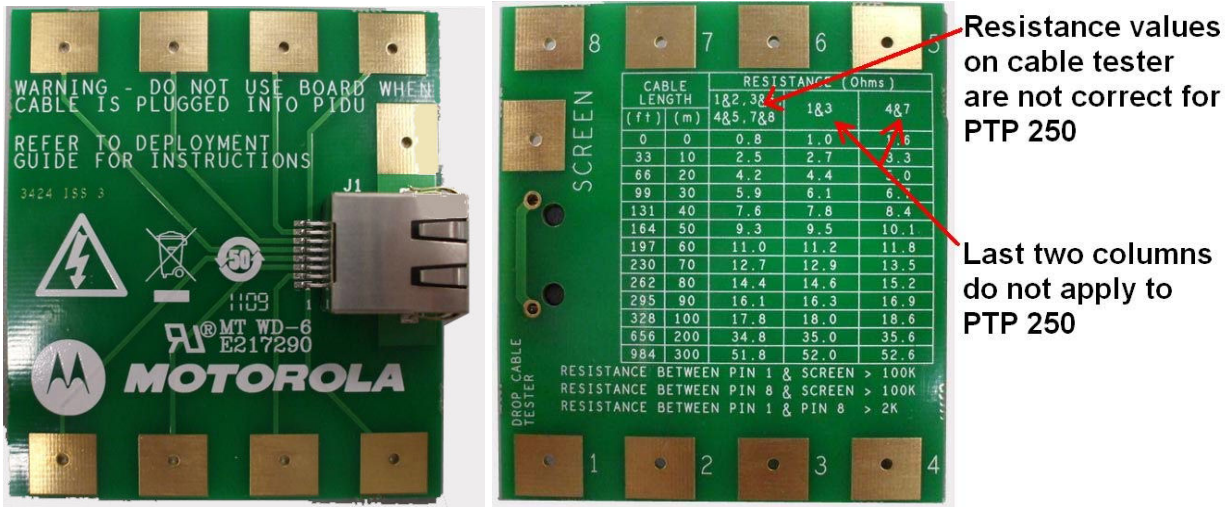
Figure 8-4 Drop cable tester (front and back views)
