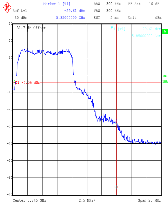
Title: Orthogon EUT: 58XX, FCC Part 15.247, Upper Band-Edge. Comment A: 45349JD01_FCC_P15-247_Top_Channel_16-QAM_Vertical_012 Date: 16.SEP.2003 09:49:46
