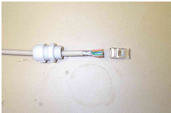
Step 3: Arrange conductors as shown in Figure 13 and cut to length
