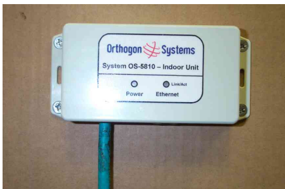
Step 1: Fix the IDU to the wall using the lugs provided.
