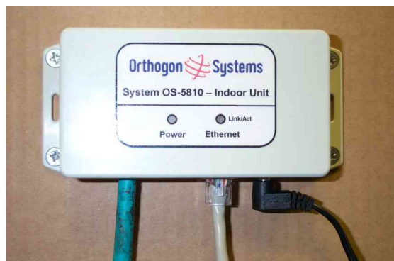
Step 2: Connect the DC power and LAN connection
