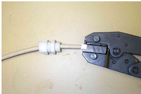
Step 4: Insert conductors and crimp
