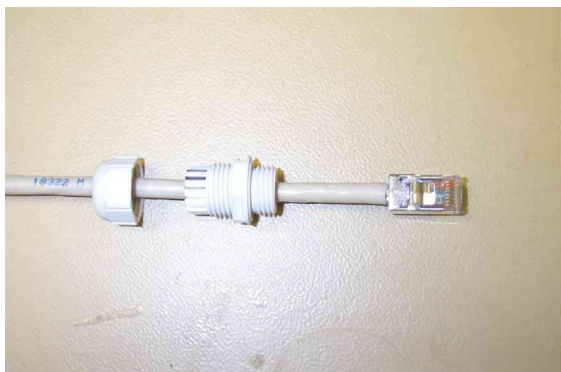
Figure 11 - Completed ODU connector
