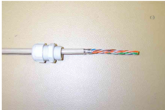
Step 2: Strip the outer insulation
