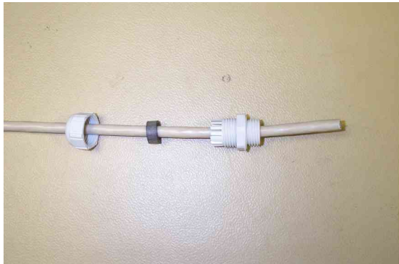
Step 1: Assemble gland on cable as shown
