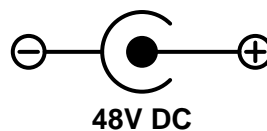
Figure 30 DC Connection Diagram
