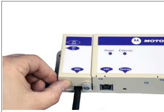
Step 3: Replace the cover and secure with the retaining screw
