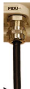
Step 4: Screw on the clamping nut and tighten (Do not over tighten – see Figure 19 )
