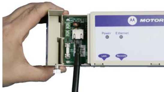
Step 2: Plug in the ODU into the PIDU Plus Cable ensuring that it snaps home
