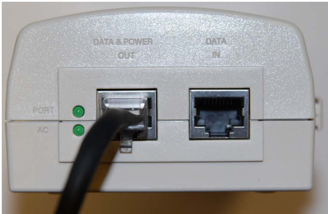
Figure 5-13 PoE power supply connected to LPU-PoE cable
