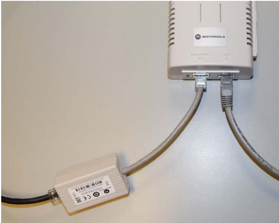
Figure 7-13 Using the reset plug
