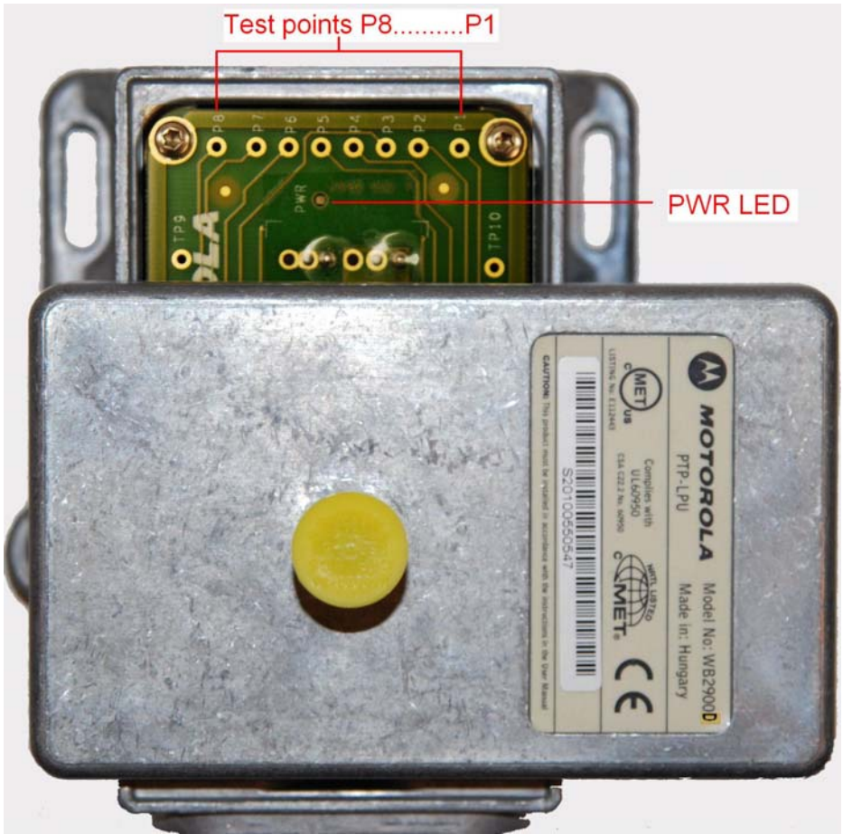
Figure 8-3 PTP LPU test points and PWR LED
