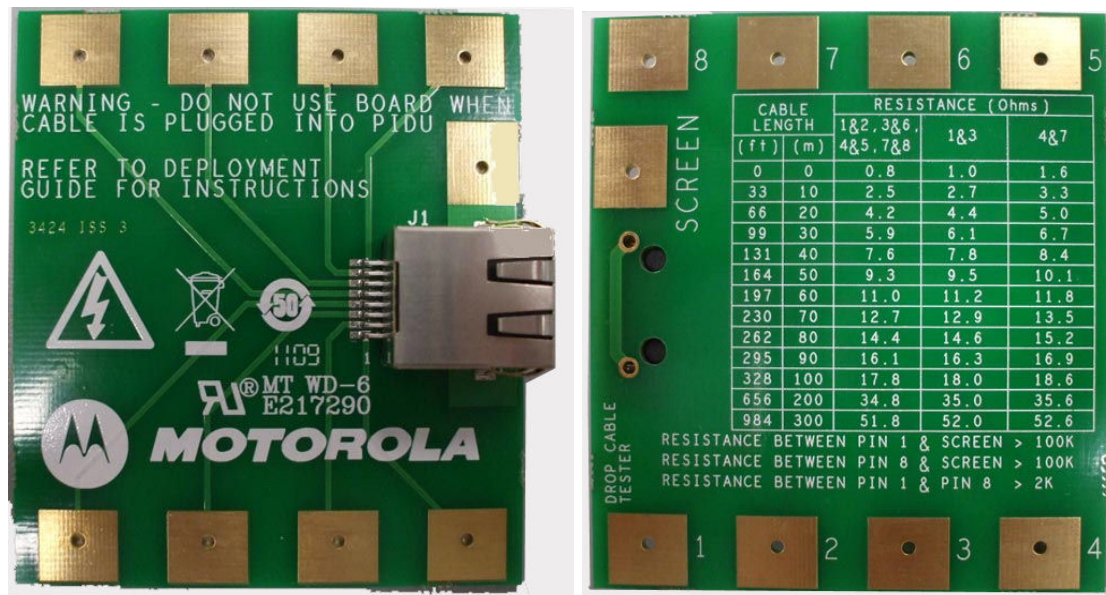
Figure 8-4 Drop cable tester (front and back views)
