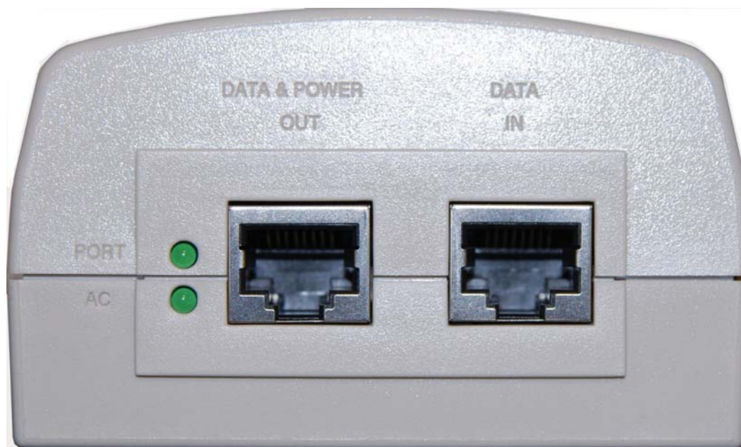
Figure 1-7 PoE power supply interfaces
