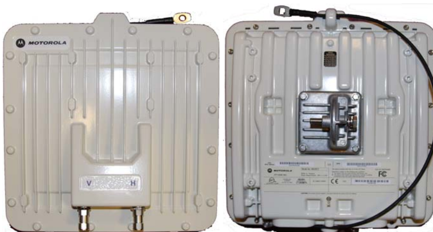
Figure 1-3 Connectorized ODU (front and rear views)
