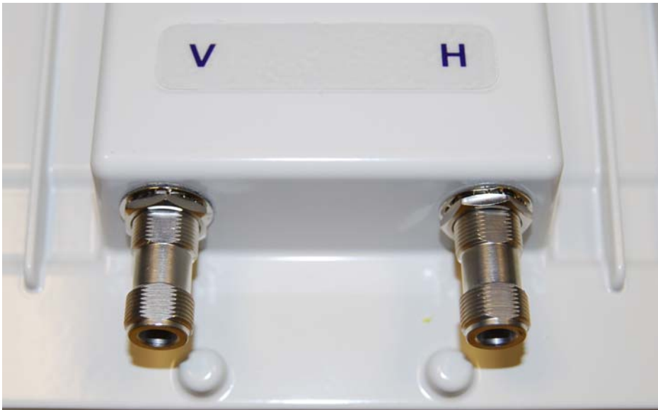
Figure 1-5 Connectorized ODU antenna interfaces
