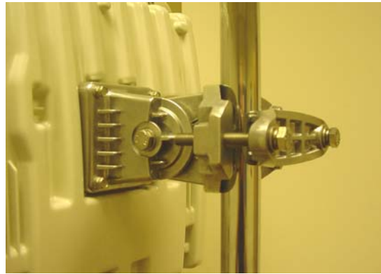
Step 2: Mate the unit to the bracket together and tighten the nut and bolt.
