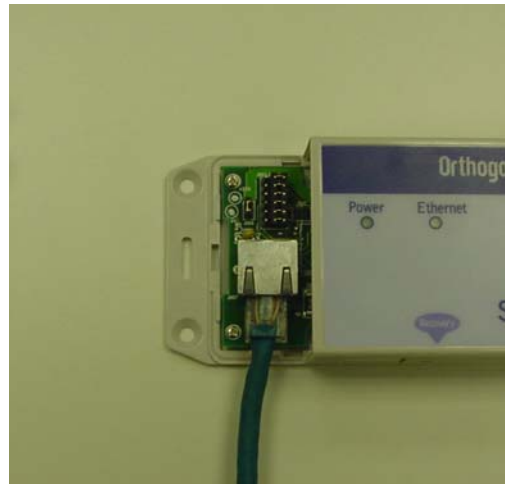
Step 2: Plug in the ODU to SPIDU Cable ensuring that it snaps home
