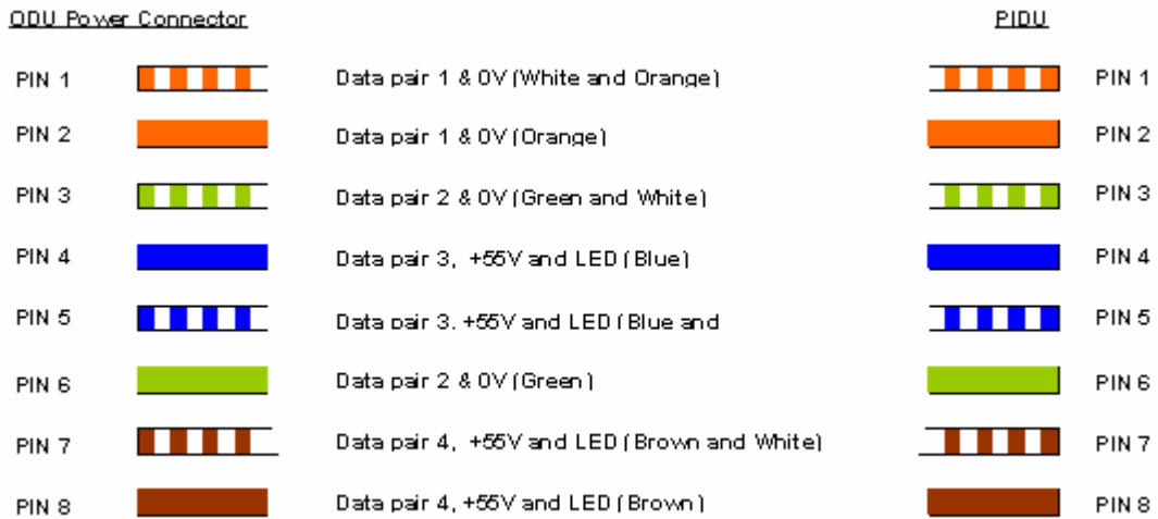
Figure 5-20 Cable connection diagram (T568B color coding)
