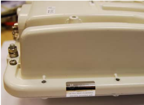
Figure 6-62 Tamper evident label on side edge of ODU
