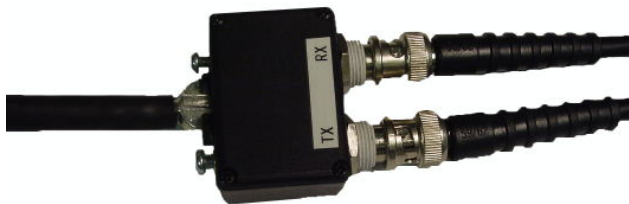
Figure 5-24 Example of a Balun
