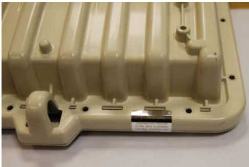
Figure 6-63 Tamper evident label on top edge of ODU
