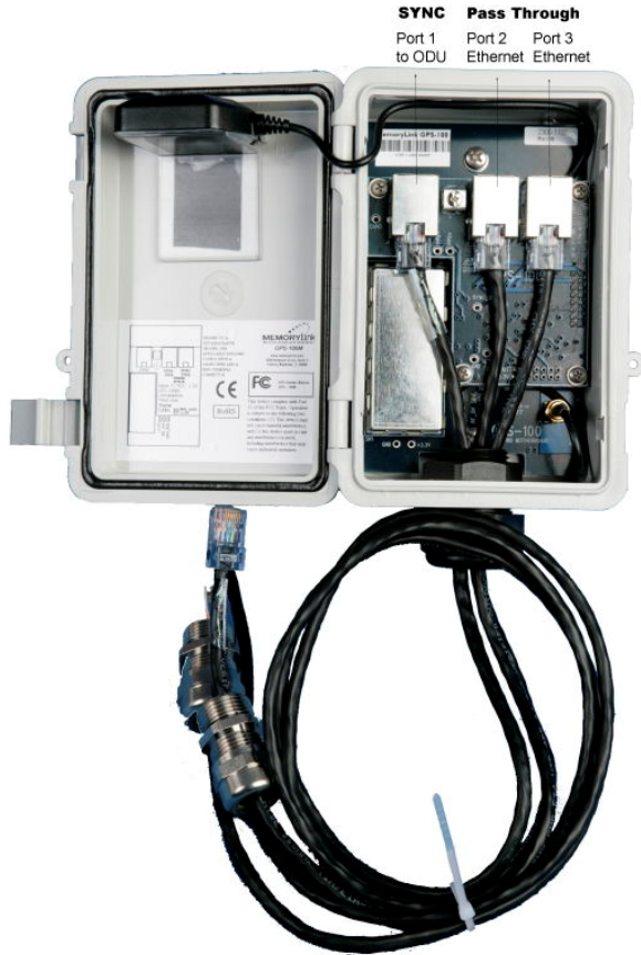
Figure 5-8 UltraSync unit connections
