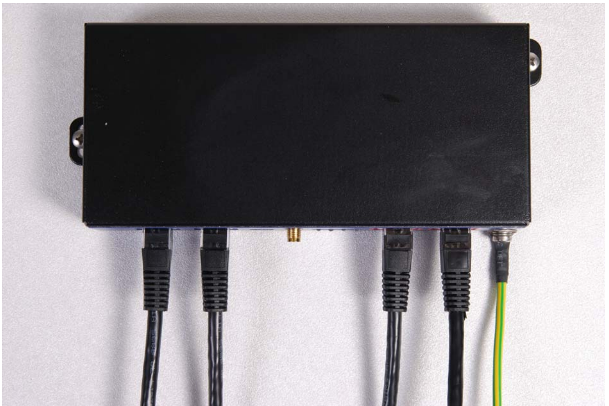
Figure 5-15 PTP-SYNC mounted on wall
