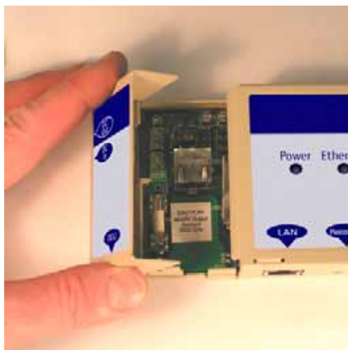
Step 1: Undo the retaining screw and hinge back the cover.
