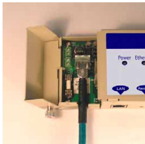
Step 2: Plug in the ODU to PIDU Plus Cable ensuring that it snaps home
