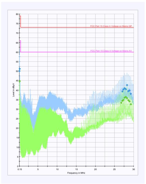
Note: Although the limits shown on this plot are of FCC Part 15 Class A, the limits on the results table shown on the previous page are of FCC Part 15 Class B
