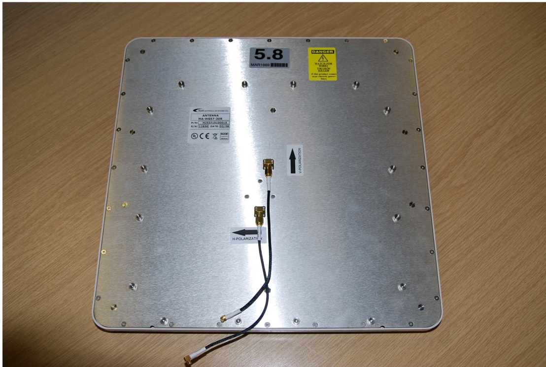
Figure 10: MARS Inc Antenna rear view, showing flying lead interconnects to radio.
