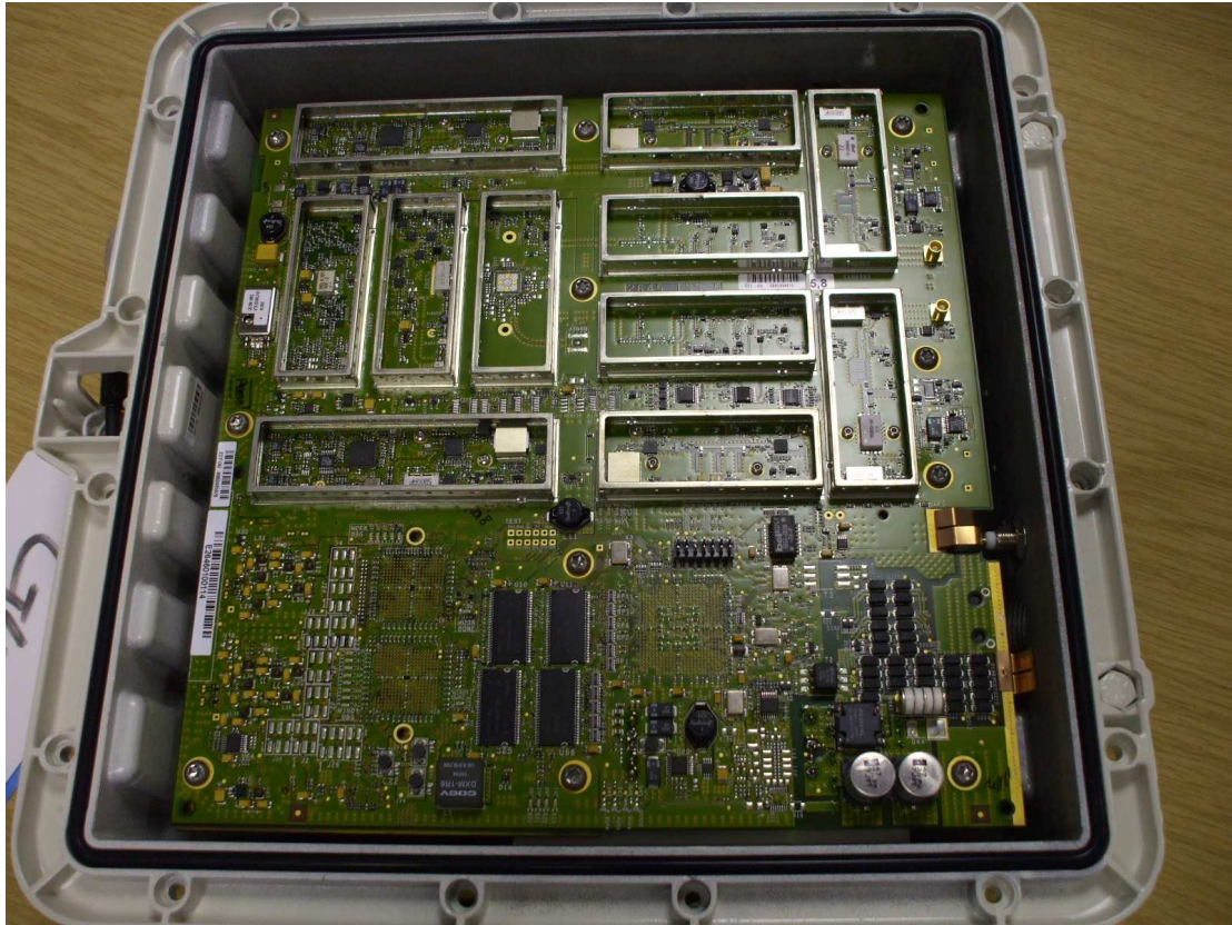
Figure 3: PTP5xx00 with cover plate and screening cans removed to show internal assembly.
