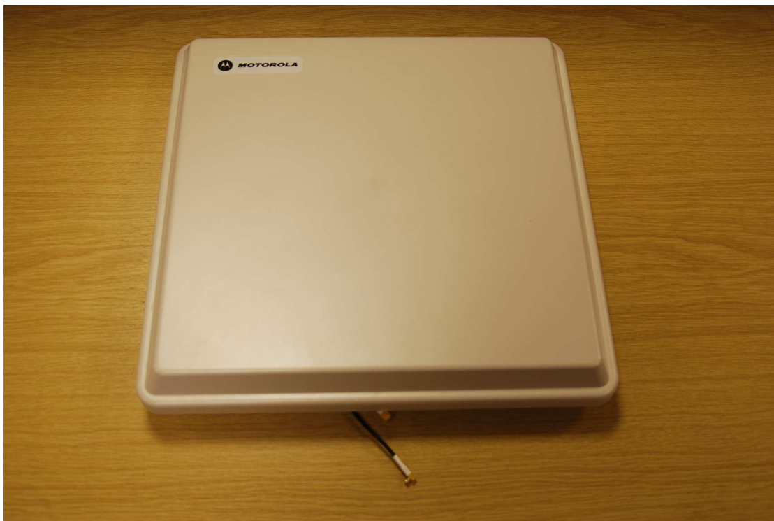
Figure 12: MARS Inc Antenna used for both 5.4 and 5.8GHz Integrated antenna versions, front view of radome.
