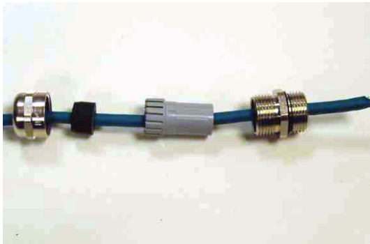
Step 1: Assemble gland on cable as shown
