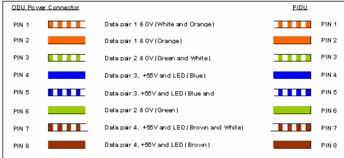
Figure 137 - Cable Connection Diagram (T568B Color Coding)
