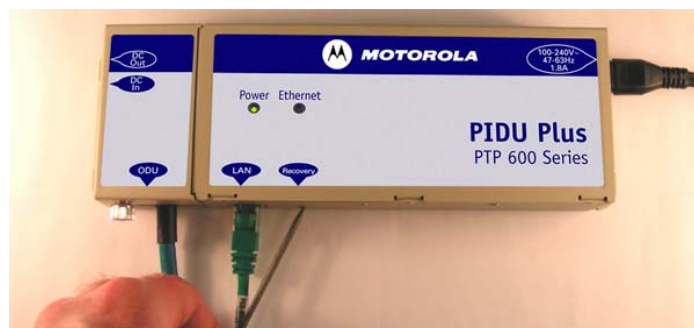
Figure 5 – PIDU Plus Recovery Switch Location
