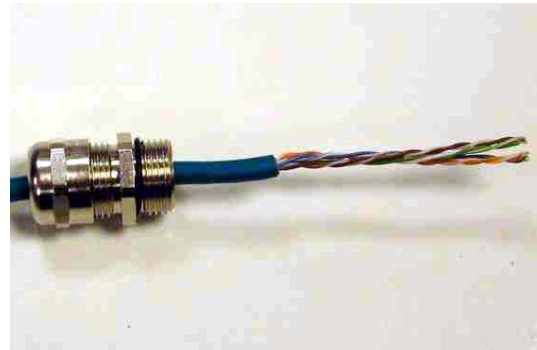
Step 2: Strip the outer insulation
