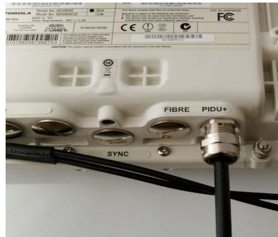
Step 4: Screw on the clamping nut and tighten
