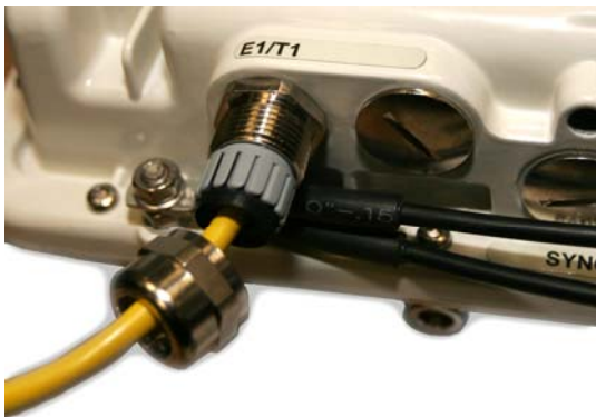
Step 3: Screw in the body of the weather proofing gland and tighten
