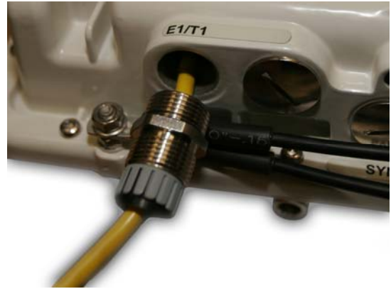
Step 2: Insert the RJ45 connector making sure that the locking tab snaps home
