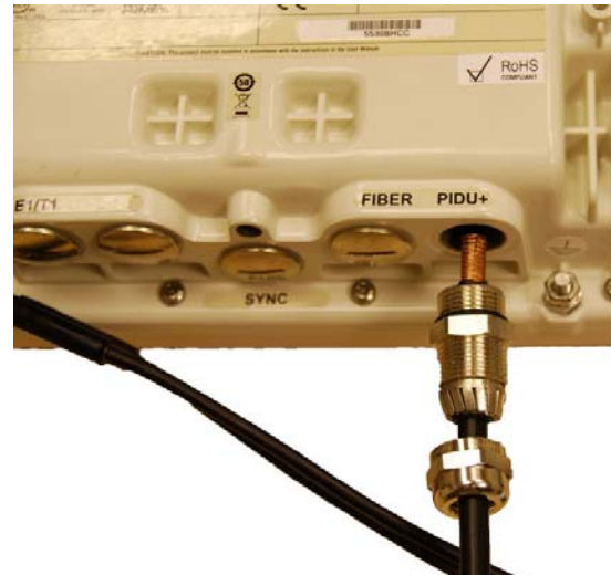
Figure 39 - Connecting the PIDU+ to the ODU
