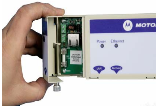
Step 1: Undo the retaining screw and hinge back the cover.
