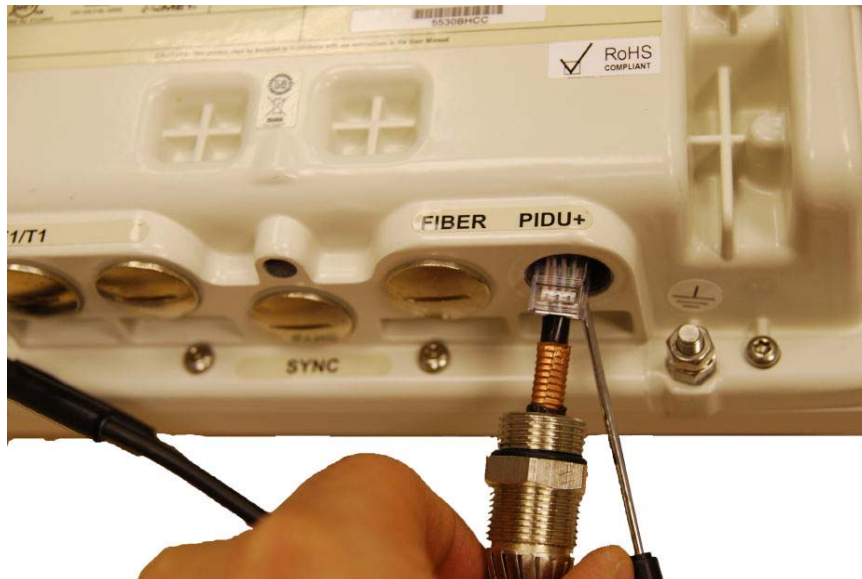
Figure 40 - Disconnecting the ODU
