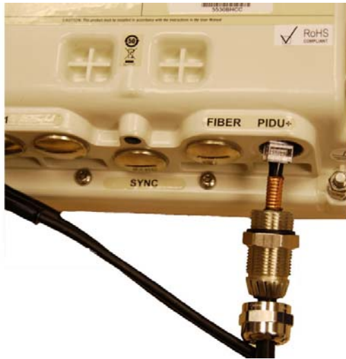
Figure 39 - Connecting the PIDU+ to the ODU
