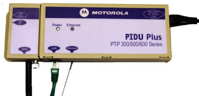
Figure 5 – PIDU Plus Recovery Switch Location
