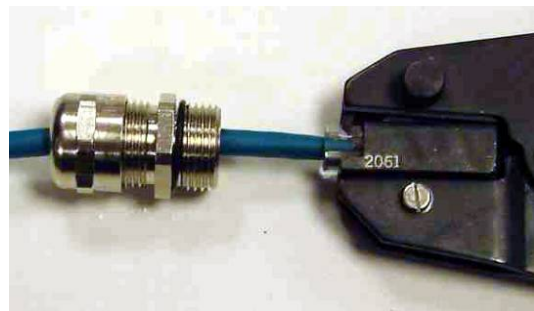
Step 4: Insert conductors and crimp
