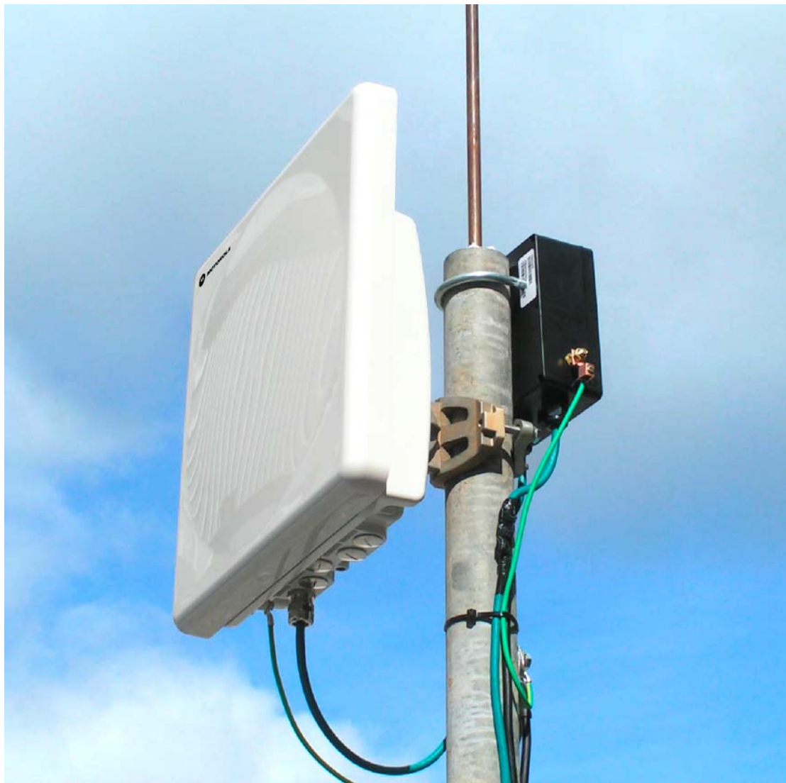
Figure 2 - PTP 400 Series Bridge Outdoor Unit (ODU)
