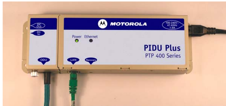
Figure 3 - Power Indoor Unit (PIDU Plus) – PTP 400 Series
