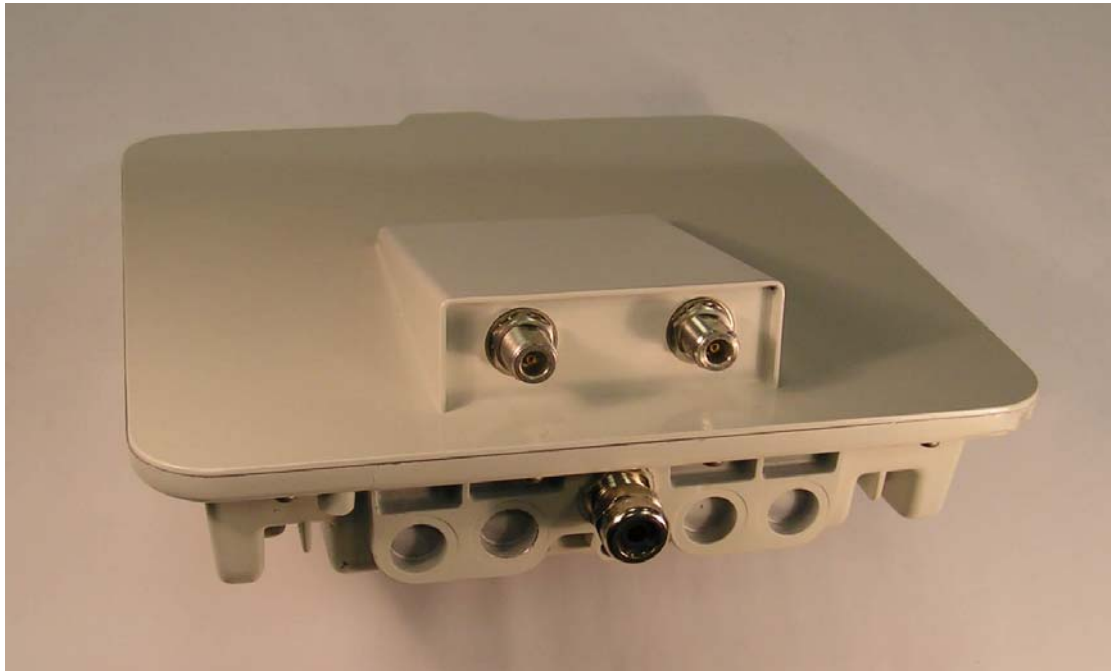
Figure 81 - Connectorized version of the PTP 400 Series bridge Outdoor Unit
