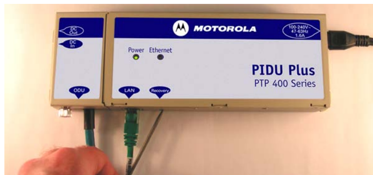
Figure 4 - PTP 400 Series Bridge Recovery Switch Location
