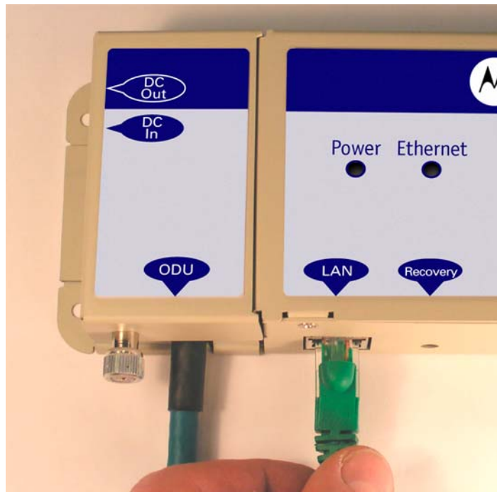
Figure 22 - Making the Network Connection at the PTP 400 Series Bridge PIDU Plus
