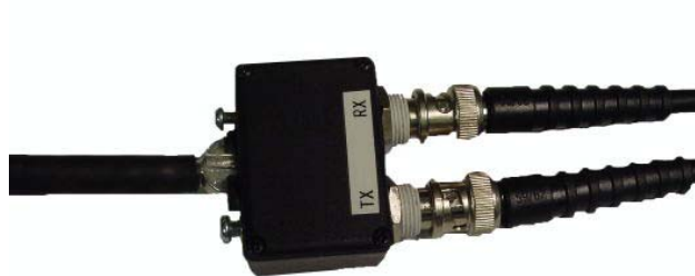
Figure 158 - Example of a Balun
