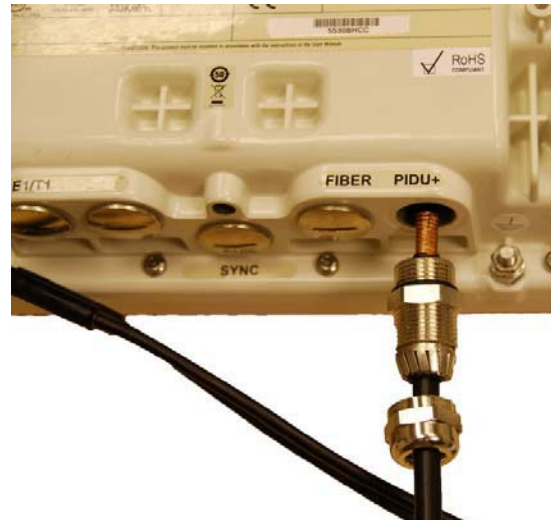
Figure 42 - Connecting the PIDU+ to the ODU
