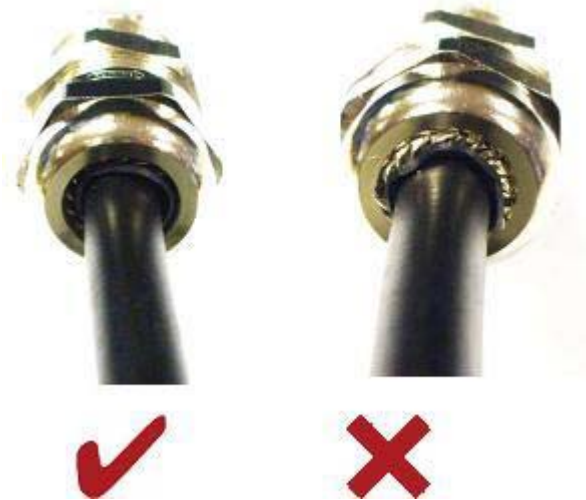
Figure 40 - Correct and Incorrect Tightening of Cable Gland
