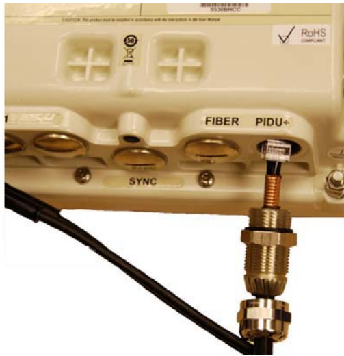
Figure 42 - Connecting the PIDU+ to the ODU
