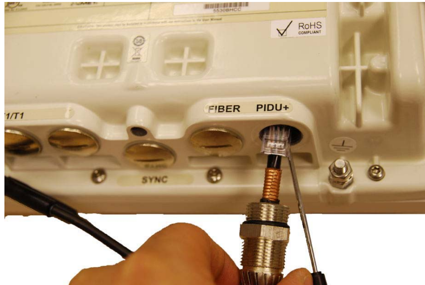
Figure 43 - Disconnecting the ODU
