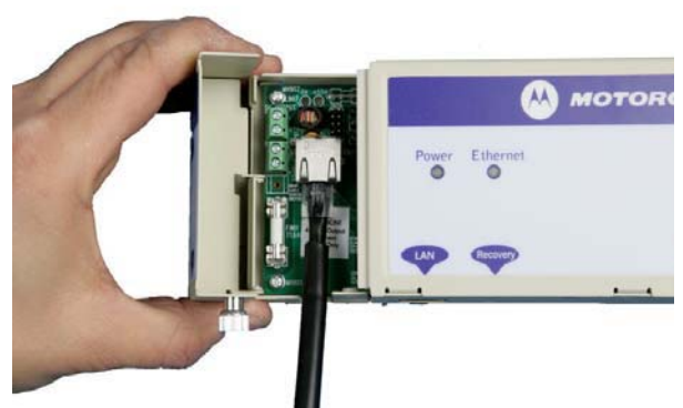
Step 2: Plug in the ODU into the PIDU Plus Cable ensuring that it snaps home
