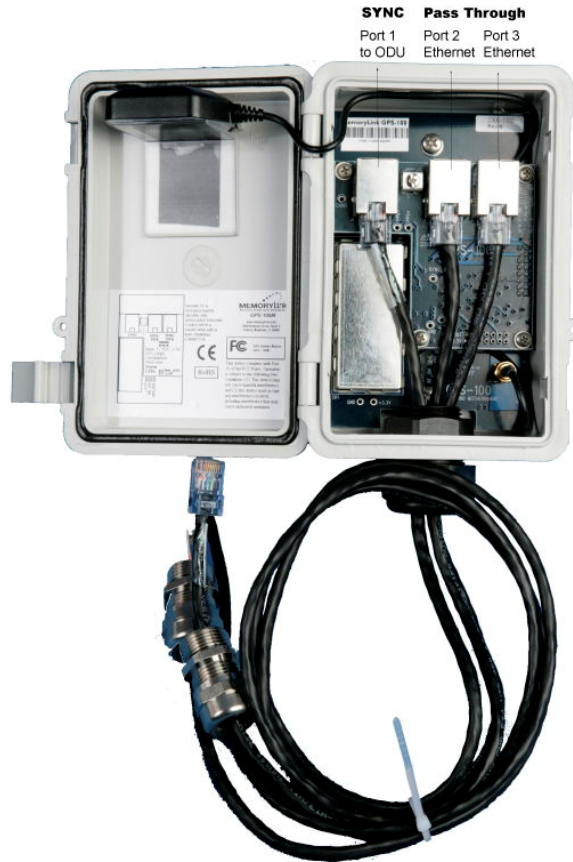
Figure 144 - GPS Synchronization Unit Connections
