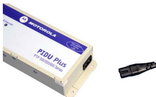
Figure 6 –PTP 300/500/600 Series Bridge PIDU Plus Power Input
