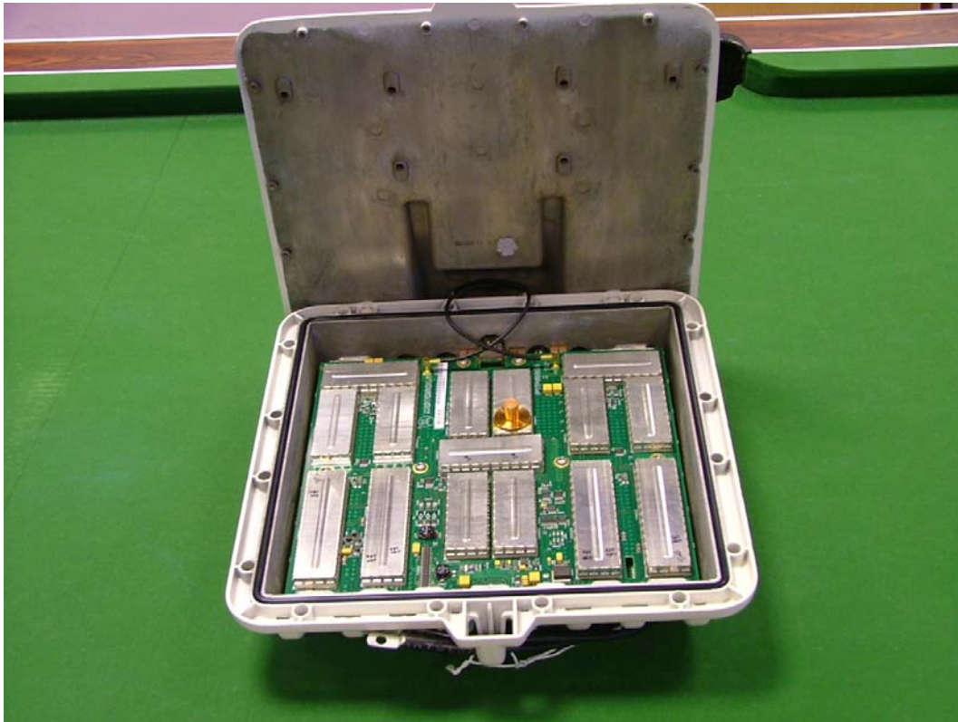
Figure 3: PTP49600 with Connector Plate removed to show internal assembly.
