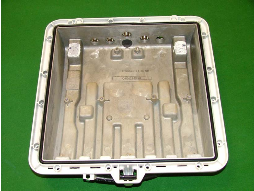
Figure 5: PTP49600 with Boards removed to show internal mechanical construction
