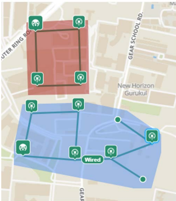
Figure 260: Unconnected zones due to isolated PoPs
