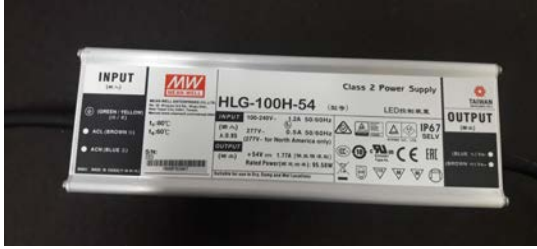
Figure 20 : Outdoor AC/DC PSU, 100W, 54 VDC
