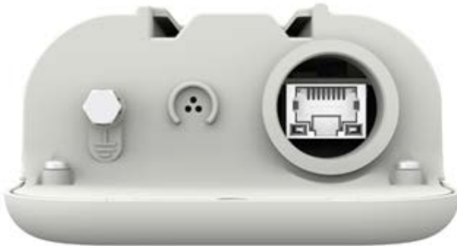
Figure 13 : External interfaces for V1000 CN
