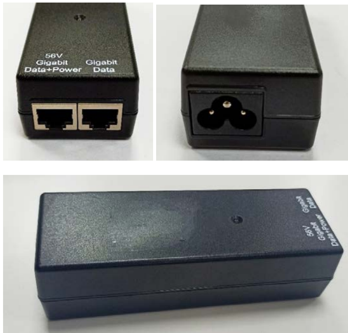
Figure 17 : PoE power supply to V1000
