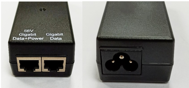
Figure 16: PoE power supply to V1000
