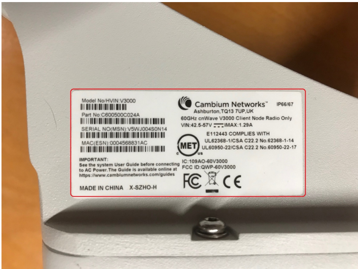
60 GHz cnWave V3000 Label Location (Close Up View)
